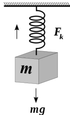
$$m \frac{d^2u}{dt^2} = mg + F_k + F_r + F_e = mg - k(L + u) + F_r + F_e = -ku + F_r + F_e,$$
